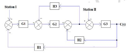
6. Analyze the given block diagram to derive the transfer function. (13) (AZ)
