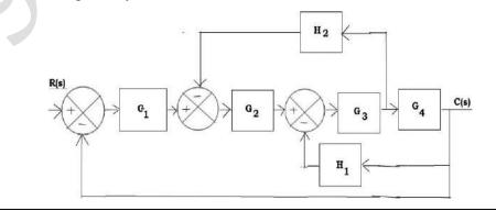
Utilize block diagram reduction rules to calculate the transfer function of the given system? (13) (E)
