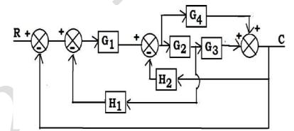
7. Examine the given system and reduce it to determine the transfer function (13) (U)
