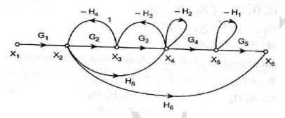
10. Demonstrate the usage of Mason's gain formula to derive the transfer function of the given graph.(13) (C)
