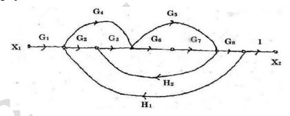
11. Apply Masons gain formula to determine the transfer function of the given signal flow graph.(13) (A)
